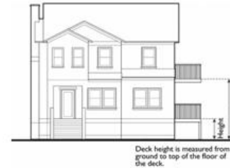
FIGURE 9-102.050-E: MEASURING HEIGHT OF DECKS
