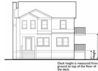
FIGURE 9-102.050-E: MEASURING HEIGHT OF DECKS
