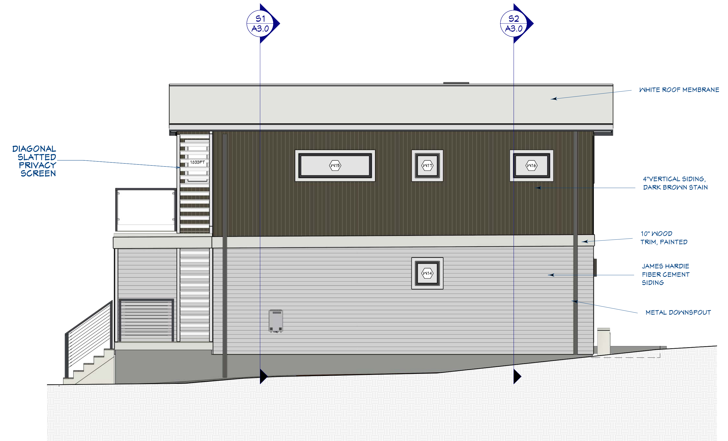
EXTERIOR ELEVATION RIGHT
