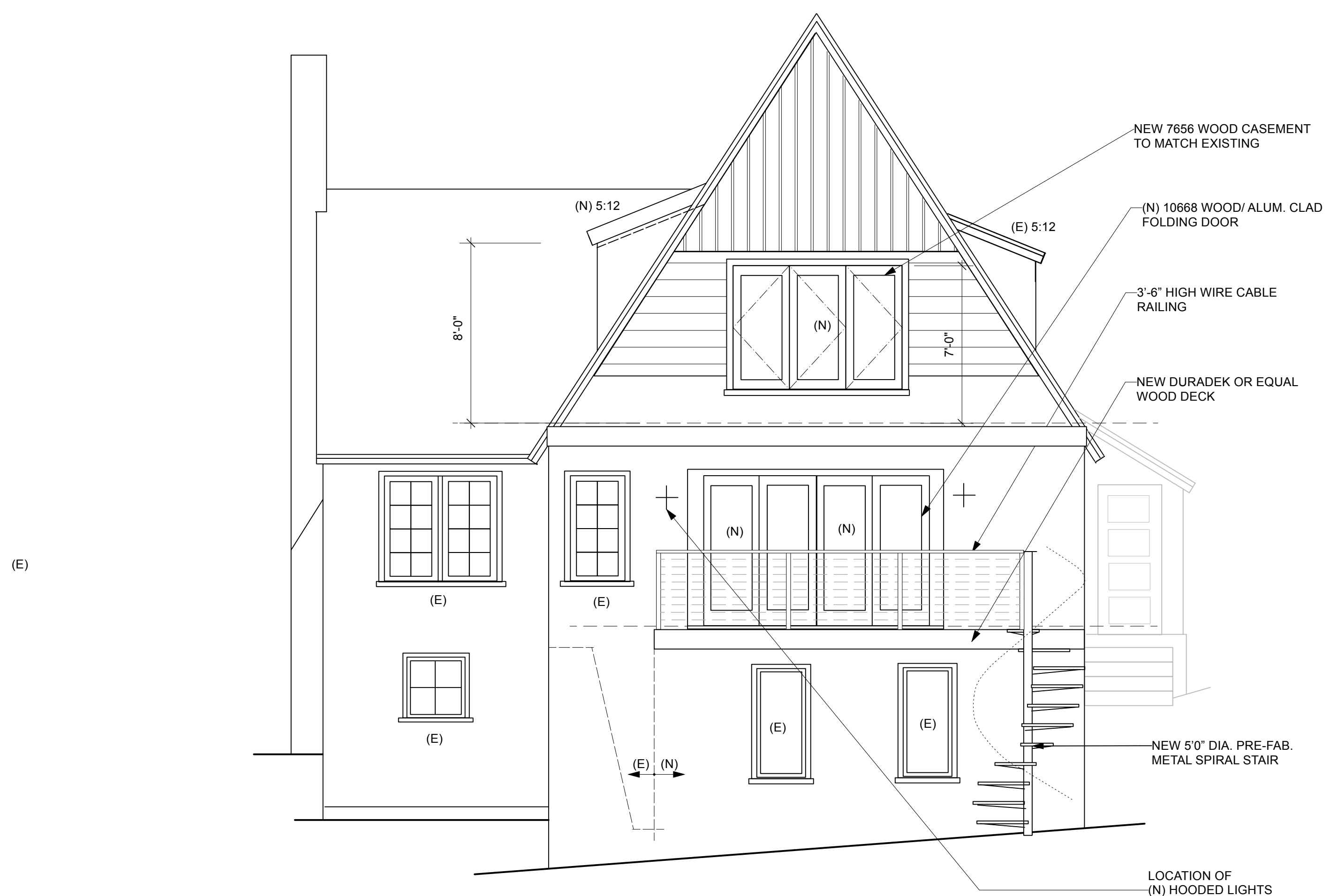
2 PROPOSED SOUTH ELEVATION 1/4" = 1'-0"
