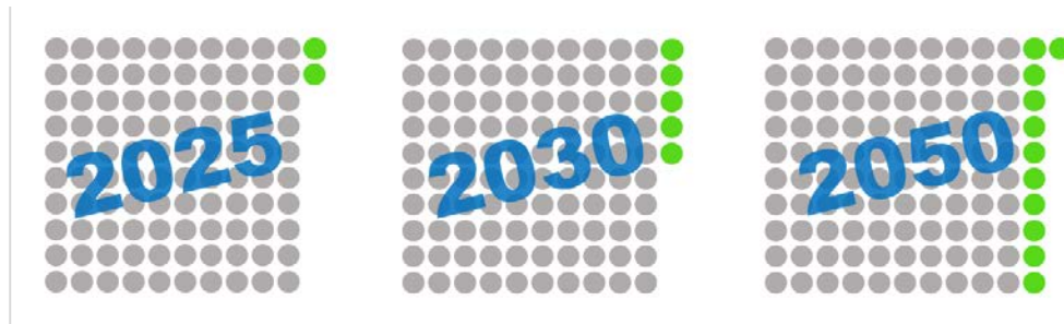
Figure 10. Comparison of New Electric Loads from EVs (Green) with Existing Consumption (Grey, based on 2017 data): Scenario 3
