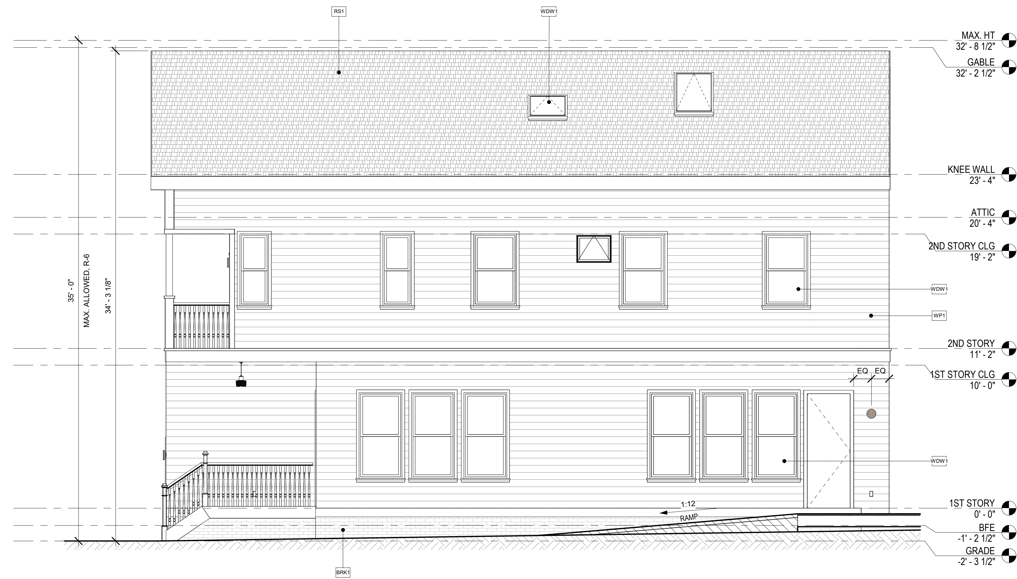
A1 BLDG ELEVATION - PROPOSED - EAST 1/4" = 1'-0"
