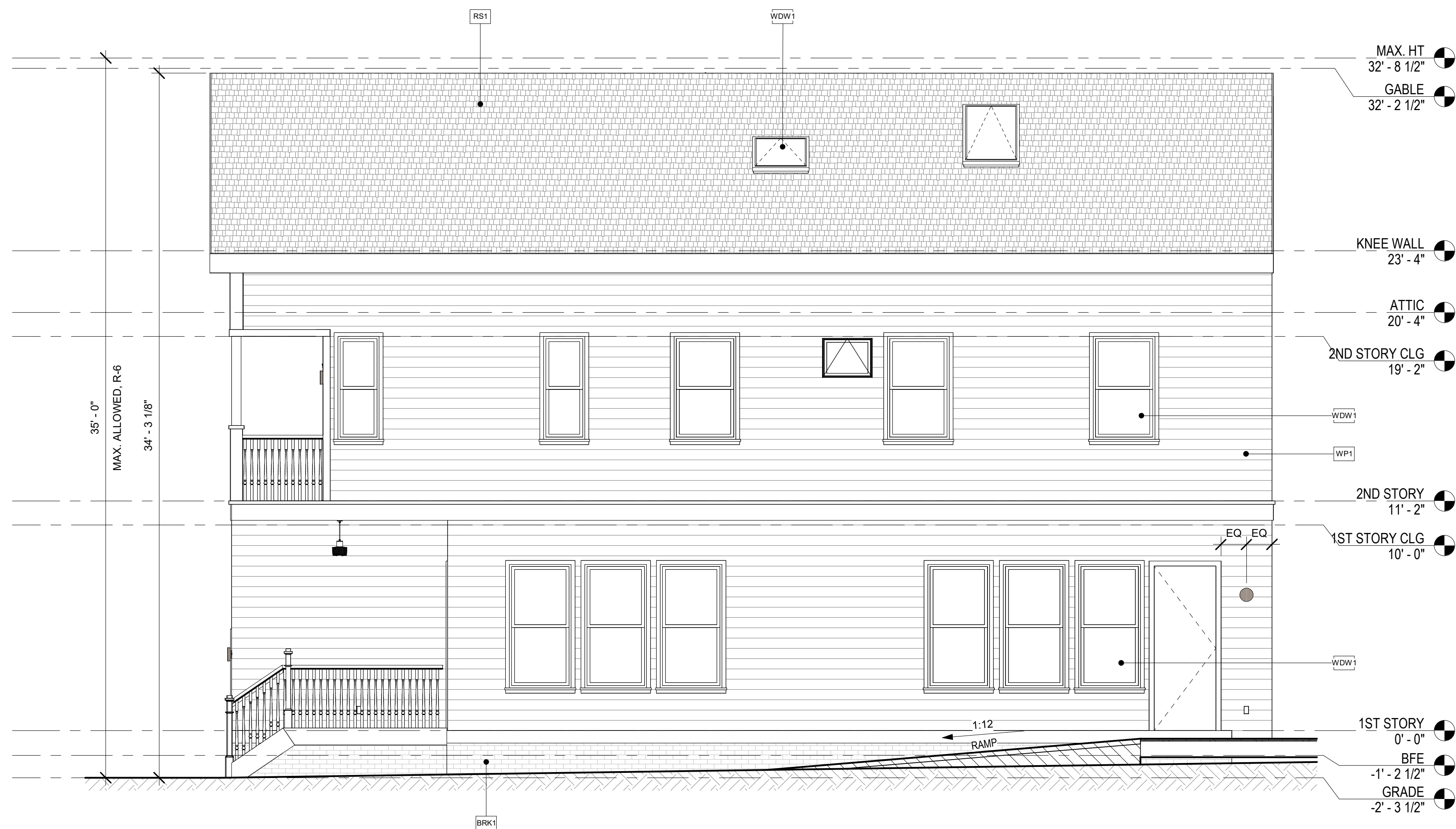
A1 BLDG ELEVATION - PROPOSED - EAST 1/4" = 1'-0"
