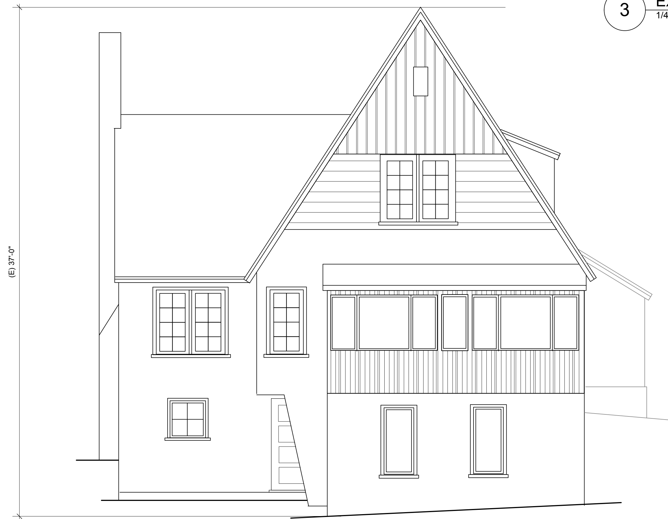
2 EXISTING SOUTH ELEVATION 1/4" = 1'-0"
