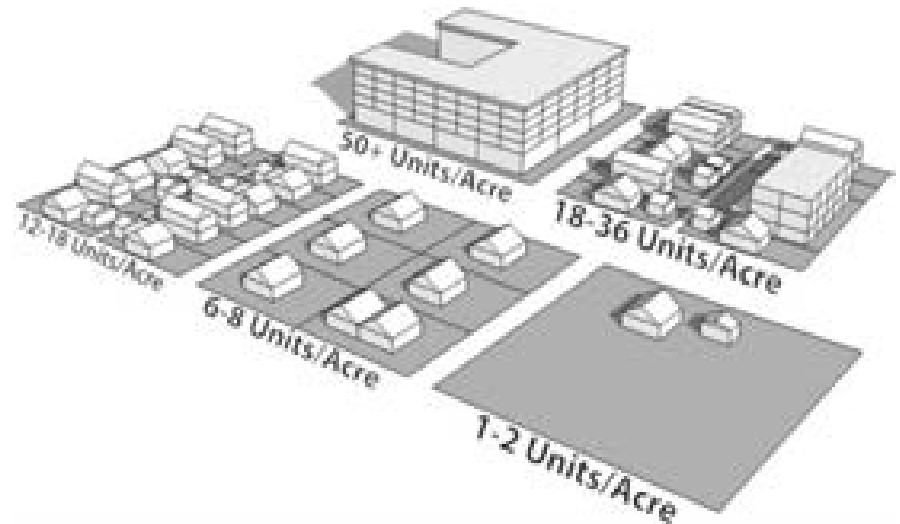
This illustration shows different densities for residential development on similarly sized lots. This graphic is intended only to show the relative differences between residential developments at various densities and does not represent a density standard for this General Plan
