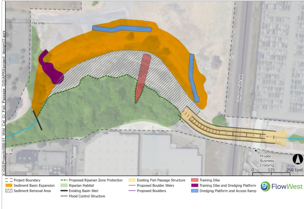
FIGURE 1 - 8: PROJECT FISH PASSAGE AND SEDIMENT BASIN ELEMENTS
