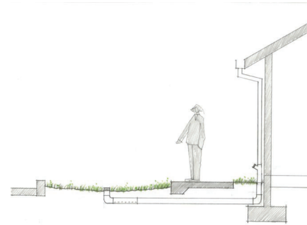
Connecting a roof leader to a vegetated area. The head from the eave height makes it possible to route roof drainage some distance away from the building.
