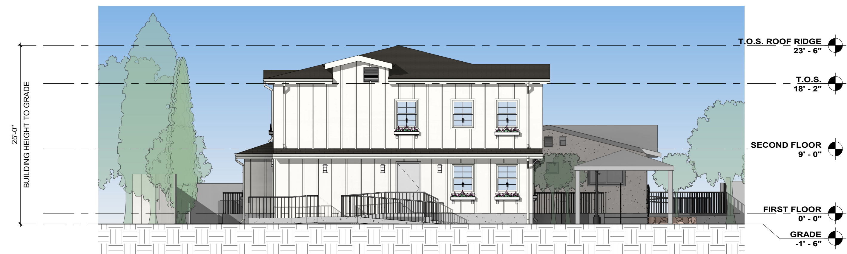
3 EXTERIOR ELEVATION - NORTH SCALE: 1/8" = 1'-0"
